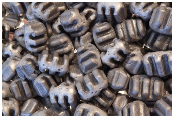
Carbon hardened geosynthetic EPS aggregate
