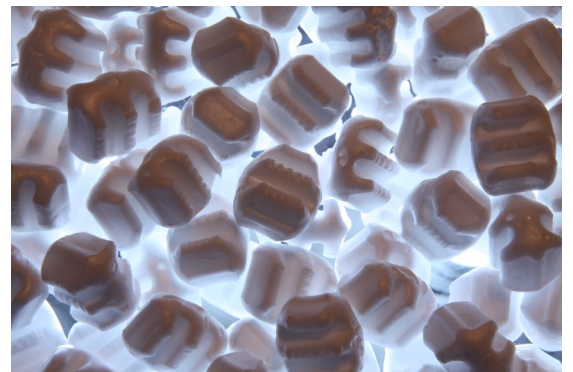
Carbon hardened geosynthetic EPS aggregate
