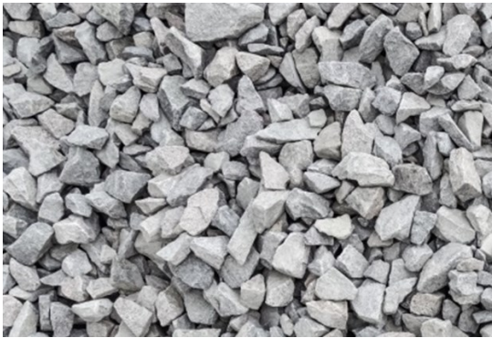
Medium grade crushed stone
