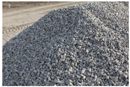
Medium grade crushed stone
